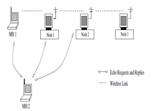
Figure 6 shows the workings of our **powerwave** program on the mobile node. The value 1.2 was derived from measur-ing the signal strength on our testbed and determining an appropriate threshold that constitutes good signal strength. Before the program starts, the following **ipchains** rule is ex-ecuted to lter out all messages (for AODV): ipchains -A input -p udp -d 255.255.255.255 1303 -s 0.0.0.0 -j DENY
