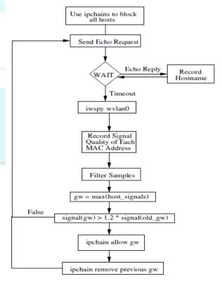
to route packets through was calculated based on previously recorded signal quality compared to current signal quality for each responding node. Note that the
